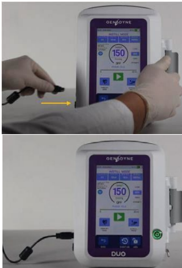
Figure 15 Connecting the Power Supply to the Device
