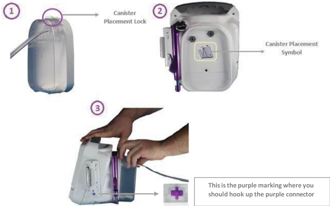
Figure 12 DUO Canister Attachment Steps
