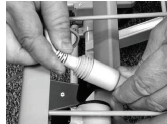
Proper Connection (completely seated)
